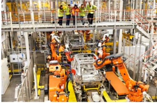
example, tyres were organised by suppliers to come off the lorry in the order they would be used on the production line to speed up production on the factory floor. It was fascinating to see how robotics were used in the production process. Barcode scanners identified the customer order as it travelled along the production line and would tell machines everything, from which seats to what engine was to be installed and what paint to spray on each car.
